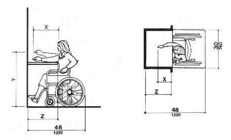
NOTE: x shall be  $\le$  25 in (635 mm); z shall be  $\ge$  x. When x  $\le$  20 in (510 mm), then y shall be 48 in (1220 mm) maximum. When x is 20 to 25 in (510 to 635 mm), then y shall be 44 in (1120 mm) maximum.
