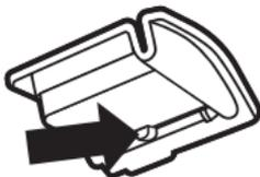
Push the flexible hook to release the sensor
